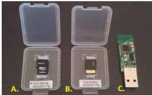
Fig. 4. ZigBee MicroSD cards (A e B) and USB Dongle CC2531 (C) [13]
